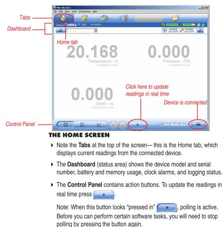
4. Software connects and displays a reading of all supported parameters.
