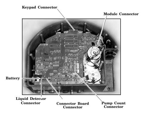
Figure 8-4 Main Circuit Board Connections
