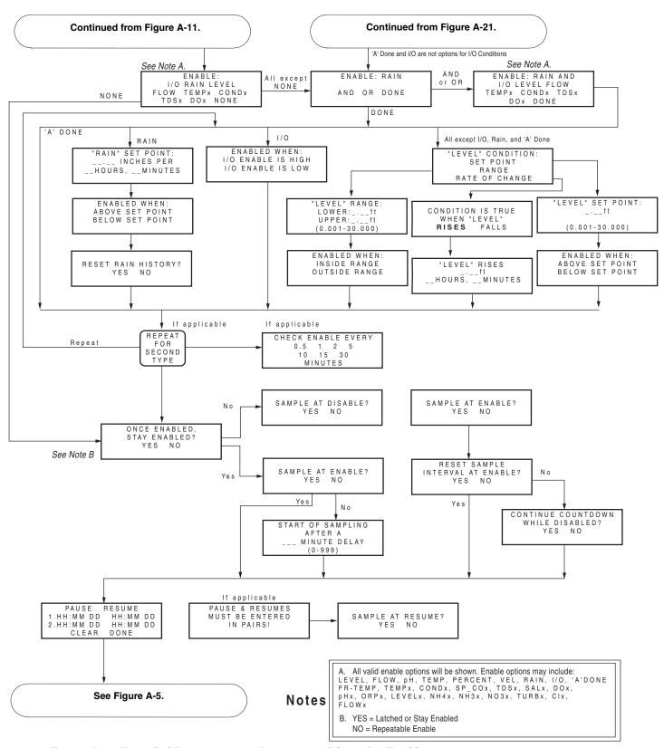
Figure A-13 Extended Programming: Programmed Sampler Enable
