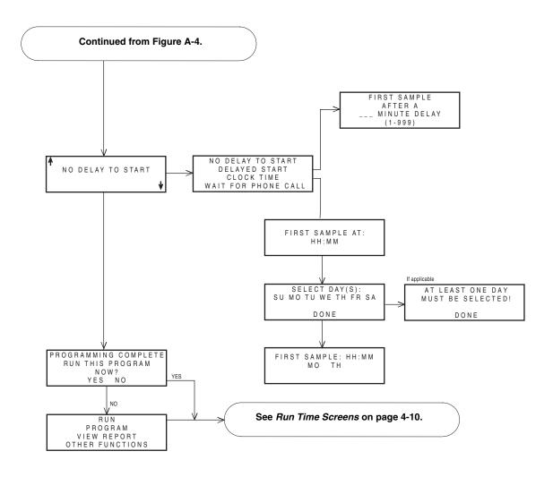
Figure A-5 Standard Programming: Quick View; Start Times
