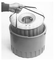
Removing Bottles From the Compact Sampler
