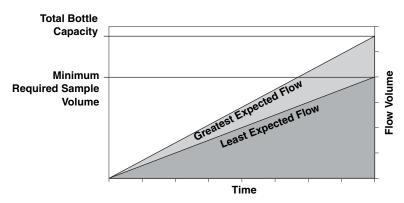
Figure 5-2 Factors Affecting Flow-Weighted Variable-Volume Samples
