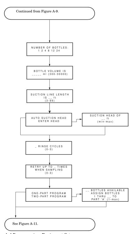
Figure A-10 Extended Programming: Equipment Setup
