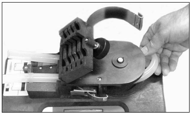
Figure 8-1 Removing and Replacing the Pump Tube
