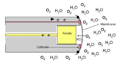
Figure 16. An illustration of an electrochemical sensor.
