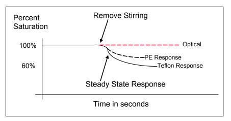
Figure 29. Flow dependence comparison graph.
