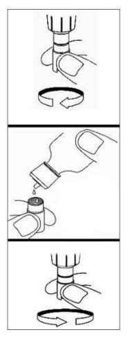
Figure 42. Sequence of drawings demonstrating a cap membrane replacement.
