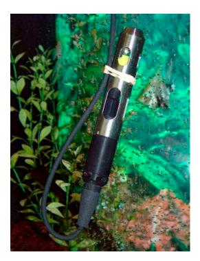
Figure 39. DO sensor inverted to avoid air bubbles bursting on the membrane surface.
