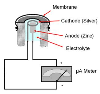
Figure 18. A simplified diagram of a galvanic sensor and circuit.
