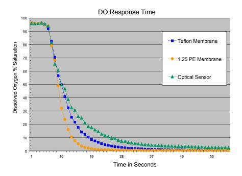
Figure 25. A graph displaying DO measurements over time for three sensors that were transferred from 100% saturated water to a zero oxygen environment.
