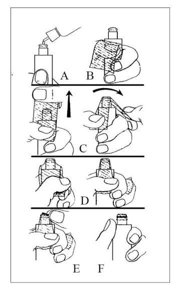
Figure 41. Sequence of drawings demonstrating a stretch membrane installation.
