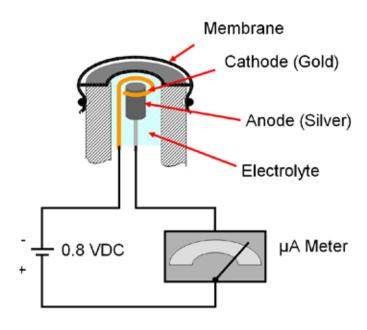
Figure 17. A simplified diagram of a polarographic sensor and circuit.
