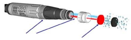
The lifetime of the luminescence is measured by the sensor and compared against a reference.
