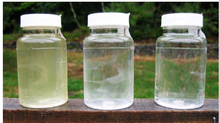
Turbidity and E. coli loads are greatly reduced with subsequent washes.
