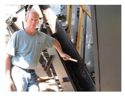
Fred holds the type of long wood chip that used to cause 'bridging' on his roller delivery system. Now that he uses metal rails to move chips this is less of a problem.
