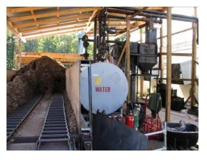
There are challenges with using waste wood versus purchasing a supply of relatively uniform wood chips from a sawmill. You have to be able to deal with branches, stumps, construction debris and other contaminant such as plastic and metal trash that can come with your 'free' fuel supply. Fred's processing system separates out the worst of the contaminants, but he needed a combustion system that could handle irregular-shaped pieces of wood and a small amount of other debris.
