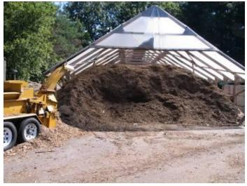
Hammermill grinder and polycovered storage that are used to process and store the wood chips.
