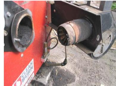
*The nozzle and fan inside the burner tend to gunk up and must be cleaned regularly*
