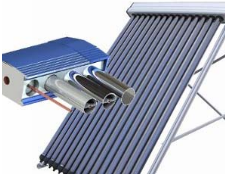
Figure 7 - Image of assembly of evacuated tube collector. The collector tubes do not directly interface with the circulated heating fluid. That fluid is carried in the manifold, and extracts heat from the bulb of the collector tubes by conduction. (Downloaded from Silicon Solar's website.)
