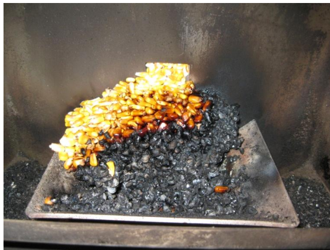
Figure 20 – ‘clinkers’ form as shell corn is combusted
