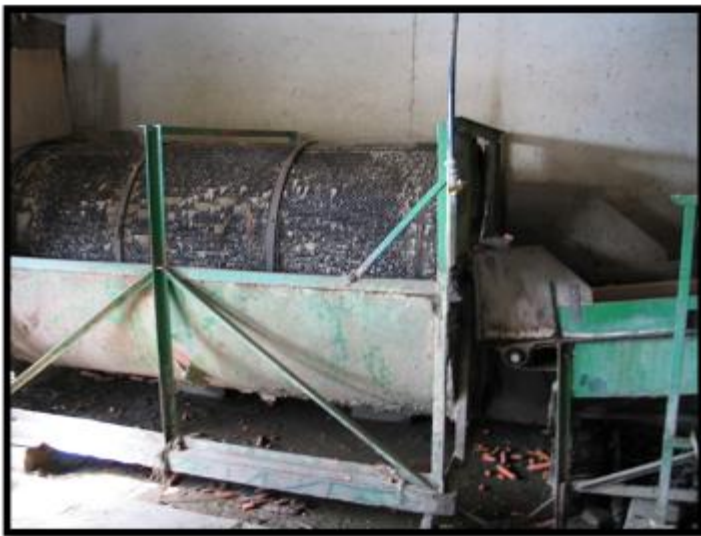
It is impossible to keep a carrot washer dirt free, but screens and catchers should be non-porous and easy to wash with high-pressure spray
