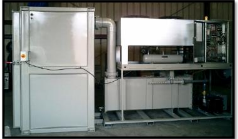
A typical 1-pallet vacuum cooling system quickly draws heat out of leafy produce tissue by forcing evaporation under vacuum pressure.
