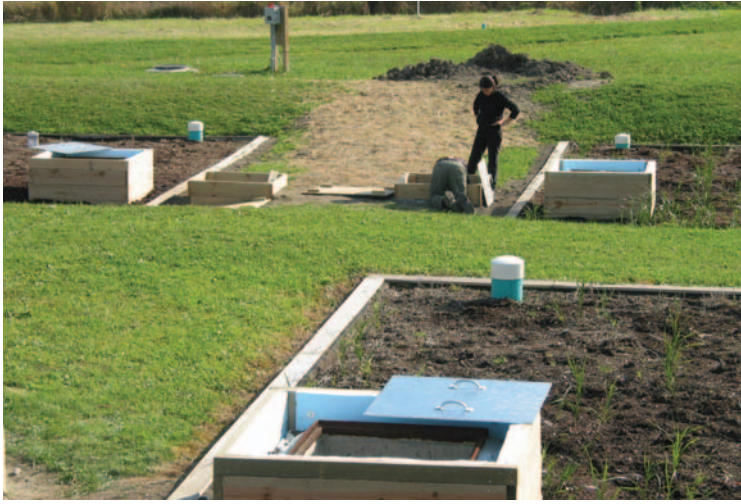
Open boxes provide access for sampling to determine the efficiency of different treatments in the constructed wetlands.
