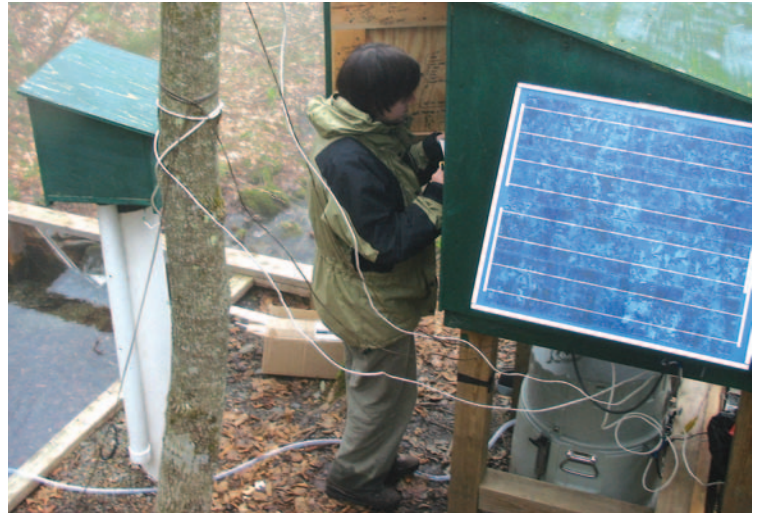
A solar panel provides power for an automated sampler that collects stream water samples at a weir.
