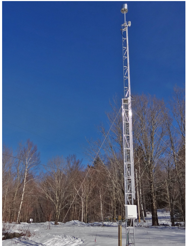
Fold-down tower used for ammonia sampling at the Underhill, VT VMC site
