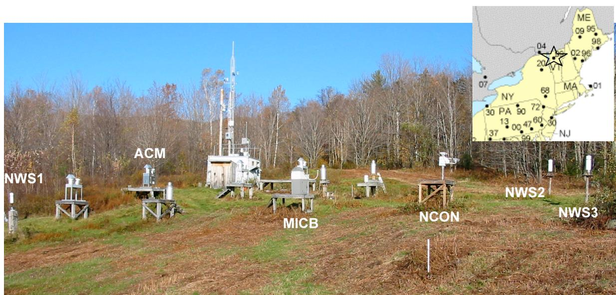
**Figure 3.** Locations of precipitation samplers at the VT99 NADP site (inset) in Underhill, VT. The NCON is farthest right (south). The MIC-B is in the center of the field. The ACM is on the left (north). The primary NWS 8-inch gage is just slightly downhill (west) of the ACM. Two additional NWS 8-inch gages were located
