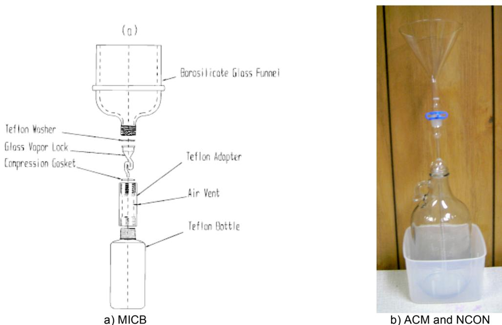
**Figure 2. a) MICB, b) ACM and NCON sample trains.**
