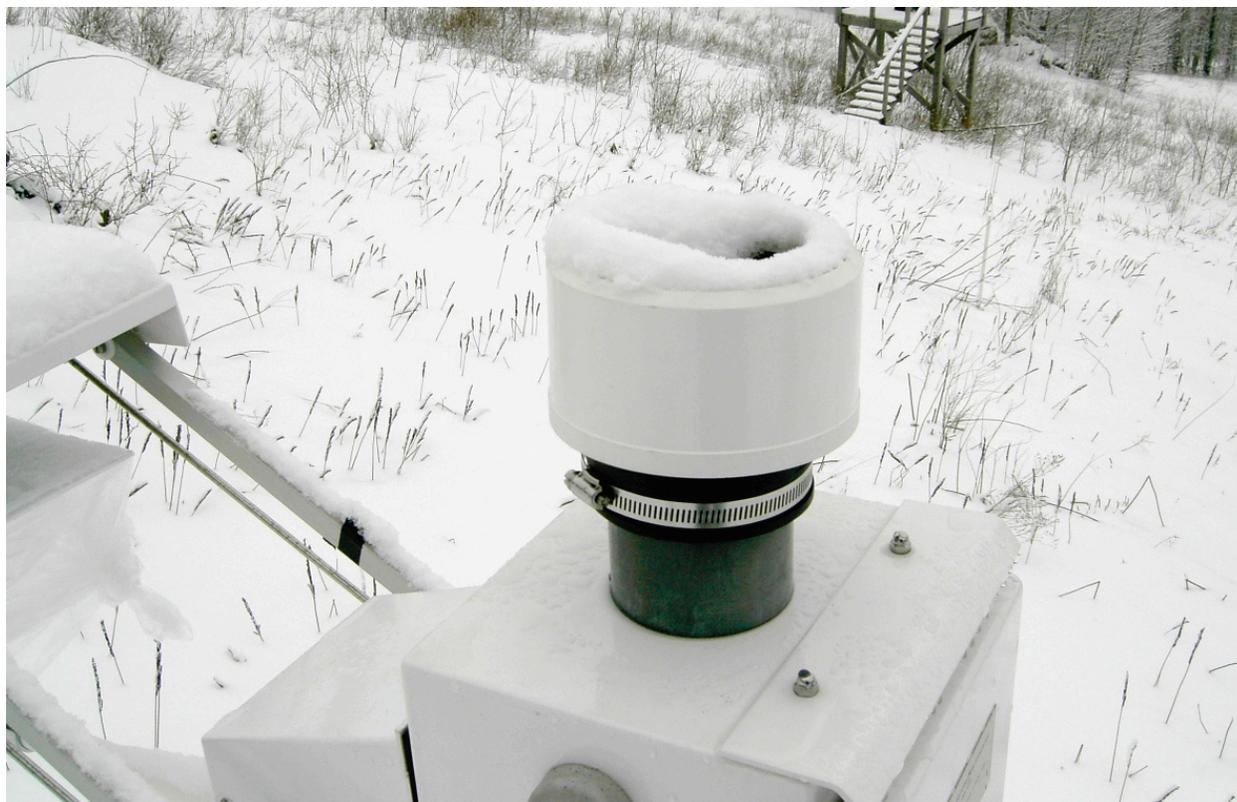
**Figure 3.** NCON sampler with unmelted snow in funnel. A portion of the snow extending above the funnel rim was knocked off when the lid closed.
