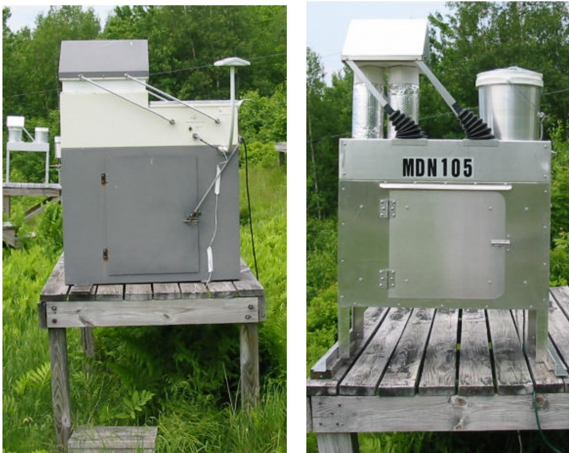
Figure. The University of Michigan (left) and Mercury Deposition Network (right) automated samplers for collecting mercury in precipitation. Moisture on a wetness-sensing element (on pole at upper right of the Michigan collector) causes the lid to automatically open, exposing a clean sample train for collection of rainfall. Site operators exchange sample trains following each rain or snow event.
