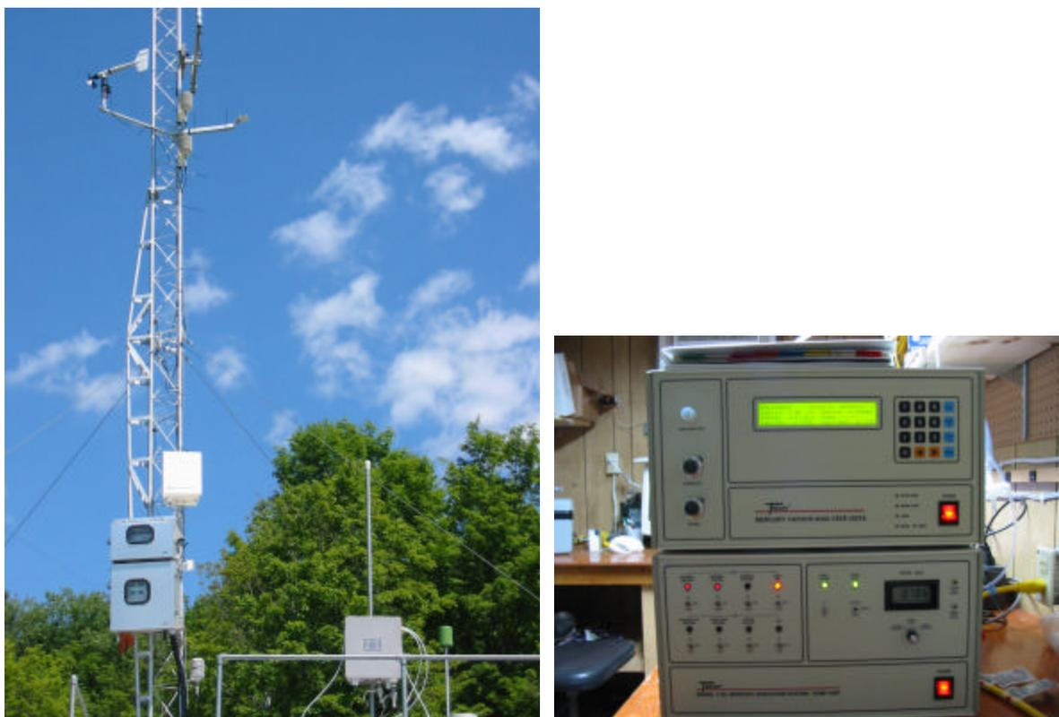
Figure. Continuous mercury speciation sampling apparatus (Tekran® 1130 and 1135 sampling heads) deployed at the Underhill Air Quality Site (left). Tekran 1130 pump module (lower right) and 2537A continuous ambient mercury vapor analyzer (upper right).
