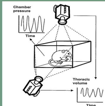
**Figure 1:** Schematic of the setup required for implementing the new invention, UVAP, in conscious mice.
