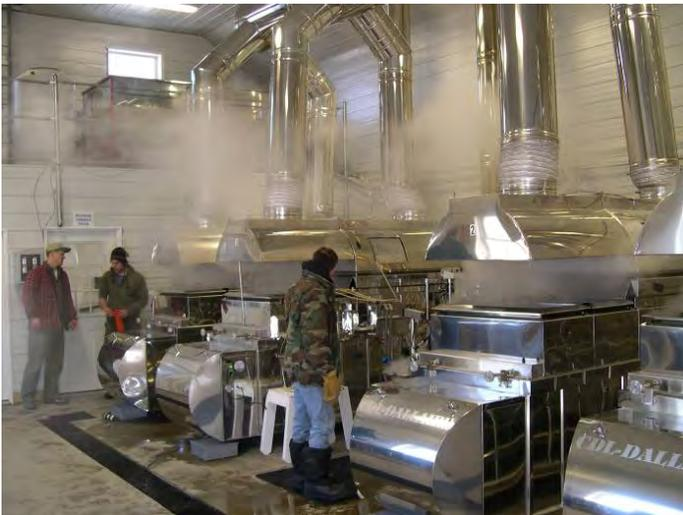
Four evaporators boiling different levels of concentrate simultaneously at the Proctor Center.
