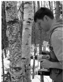
Researcher Mark Isselhardt of the PMRC prepares a sensor to measure sap pressure in birch.
