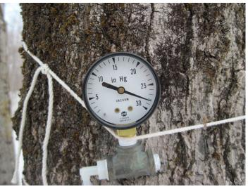
High sap yields, critical to a sugarmaker's success, are made possible by high vacuum levels. The gauge shows vacuum achieved by a new low-tech gravity collection system. Vacuum at this level was previously achieved only with a vacuum pump.
