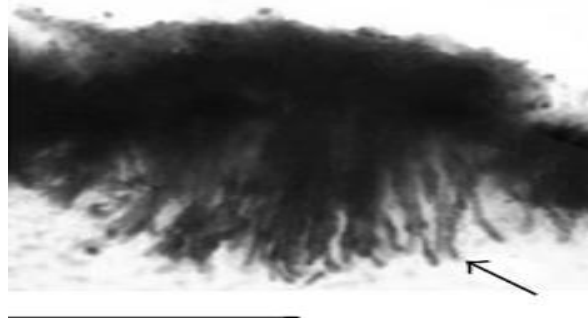
Figure 1: Hyphae penetrate the silicone of a voice prosthesis, causing it to expand and stiffen (Leonhard et al. , 2010.)
