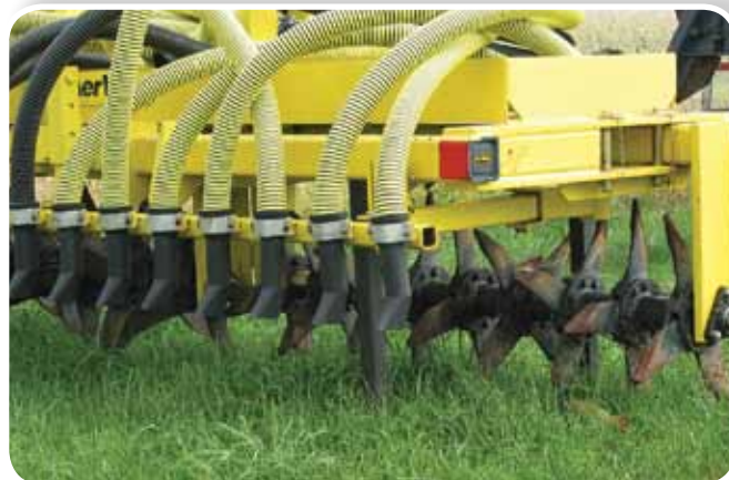
Left: Chisel injector with sweeps, which includes a disk to cut surface residue. Right: An aerator set up to band liquid manure over the injection slots. Photos originally submitted with the Journal of Environmental Quality article "Manure Application Technology in Reduced Tillage and Forage Systems: A Review," by R.O. Maguire et al. (40:292–301).
