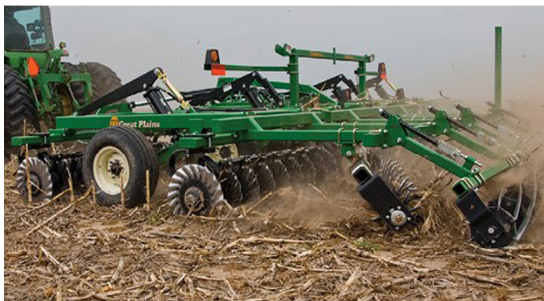
(above) Vertical tillage implement (Great Plains) with straight cutting disks, rotary harrow and rolling baskets.
