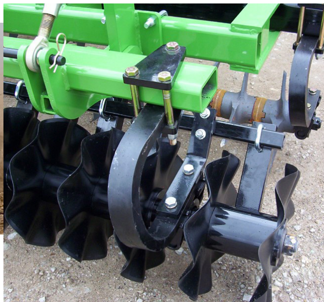
(above) Vertical tillage implement (Great Plains) with straight cutting disks, rotary harrow and rolling baskets.
