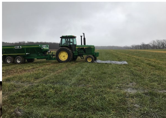
(left) Calibrating the spreading of short paper fiber lime from Casella Organics, LLC. The tractor/spreader drove over a known area – the tarp – and we weighed the material to determine the spreading rate.
