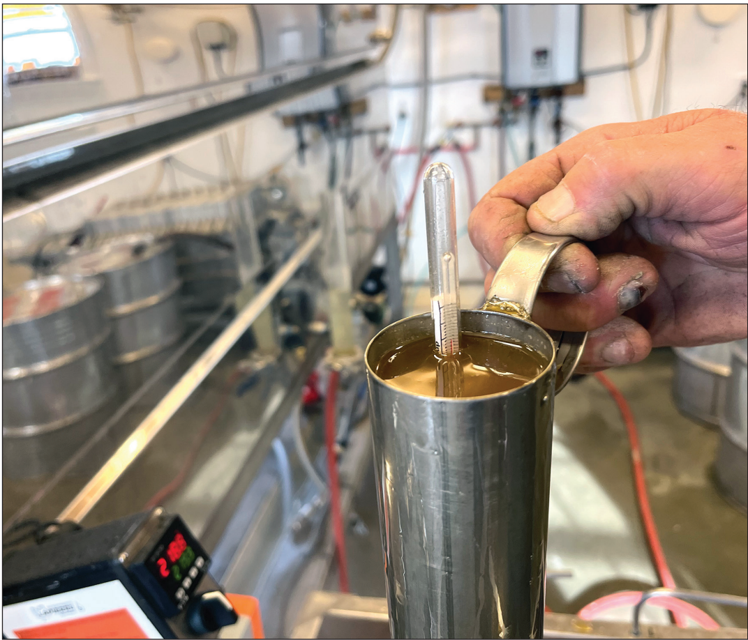
SUGARMAKERS ARE ENCOURAGED to pay close attention to density this season, using a properly calibrated hydrometer. A recent survey by UVM Ext. found that many online syrup purchases were out of density compliance in Vermont.
