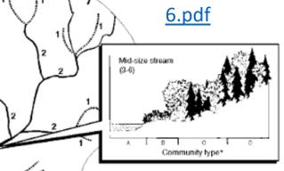
Stream orders are a simple numbering system used to classify the drainage network of a watershed. Order 1 streams are the first channels in the headwaters to exhibit a defined bed and banks. Most are only 1-2' in width. Two order 1's join to form an order 2 and so on.
