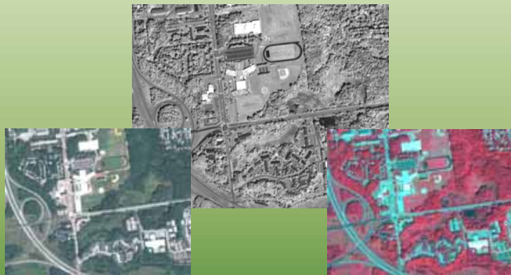
Figure 1. Natural color, panchromatic, and color infrared composite images from QuickBird satellite data
