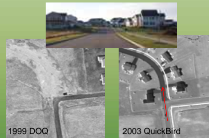
Figure 3. QuickBird satellite imagery can be used to monitor land use change over time. New housing at Barber Farms in South Burlington is evident in the QuickBird satellite data acquired in 2003 that was not present in the 1999 DOQ.
