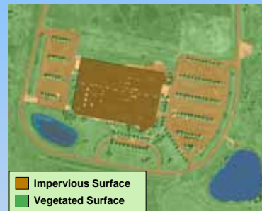
Figure 2. Impervious area map for stormwater management in South Burlington, VT derived from QuickBird satellite imagery.
