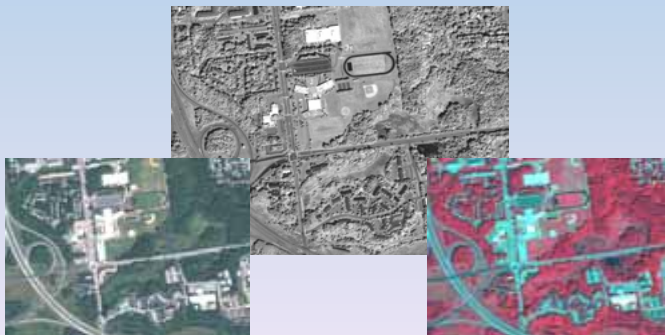
Figure 1. Natural color, panchromatic, and color infrared composite images from Digital Globe's QuickBird satellite
