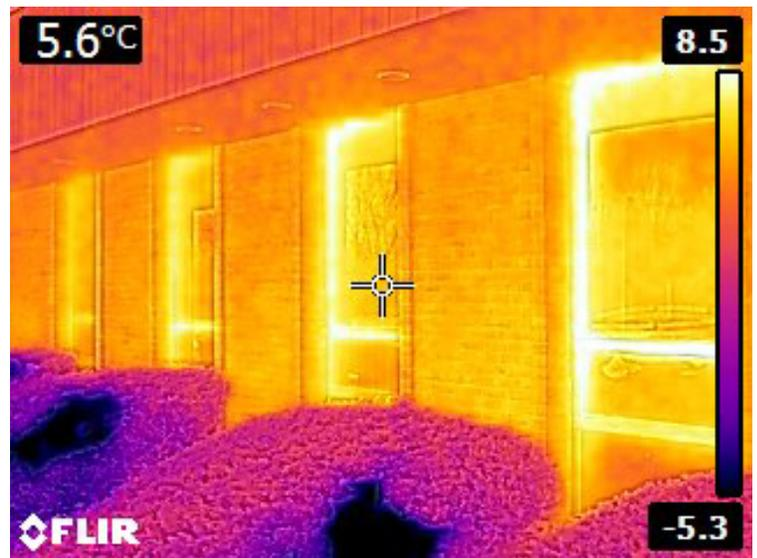
Infrared image of the Forestry Sciences Lab windows showing heat loss around window edges.
