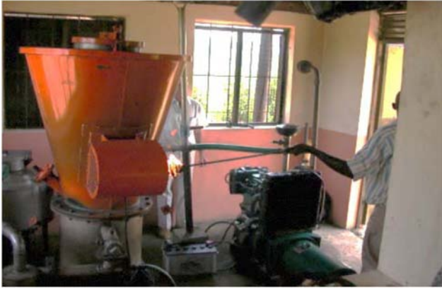
Figure 8: 10 kW dual fuel mode gasifier for electricity production
