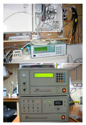
Valve Box, CO2/H2O and Hg Analyzers
