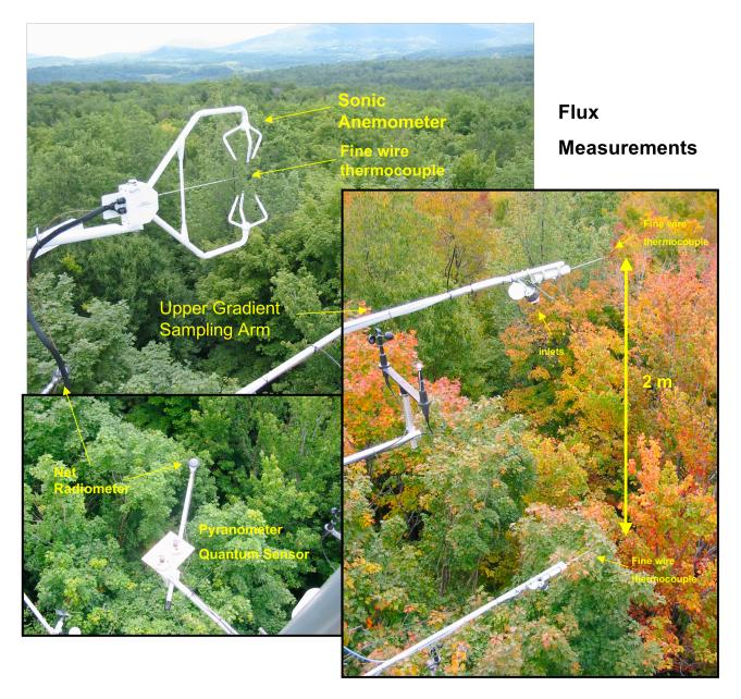
Figure 1. Configuration of inlets and sensors for the GEM flux measurement system deployed on top of the forest canopy observation tower.
