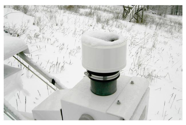
**Figure 3.** NCON sampler with unmelted snow in funnel. A portion of the snow extending above the funnel rim was knocked off when the lid closed.
