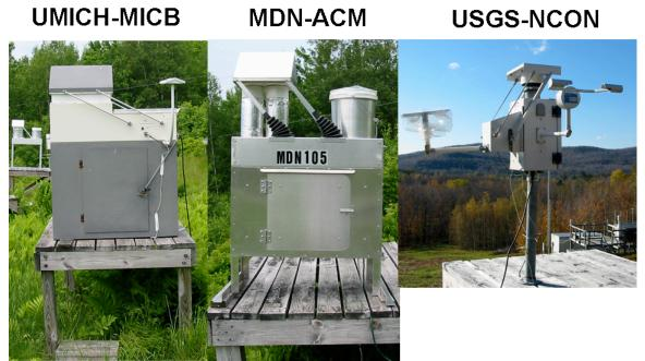
**Figure 1.** a) University of Michigan modified MIC-B collector, b) MDN modified Aerochem collector, and c) USGS NCON collector.
