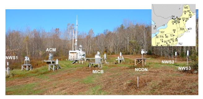
**Figure 3.** Locations of precipitation samplers at the VT99 NADP site (inset) in Underhill, VT. The NCON is farthest right (south). The MIC-B is in the center of the field. The ACM is on the left (north). The primary NWS 8-inch gage is just slightly downhill (west) of the ACM. Two additional NWS 8-inch gages were located
