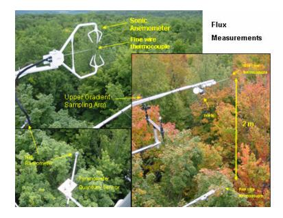
Figure. Elements of the flux measurement system deployed above the forest canopy at the VMC Canopy Research Tower in Underhill, VT.
