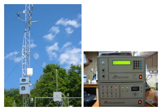
Figure. Continuous mercury speciation sampling apparatus (Tekran® 1130 and 1135 sampling heads) deployed at the Underhill Air Quality Site (left). Tekran 1130 pump module (lower right) and 2537A continuous ambient mercury vapor analyzer (upper right).
