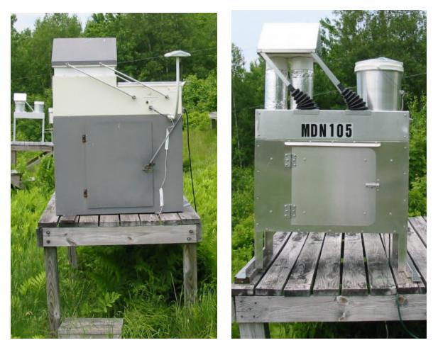
Figure. The University of Michigan (left) and Mercury Deposition Network (right) automated samplers for collecting mercury in precipitation. Moisture on a wetness-sensing element (on pole at upper right of the Michigan collector) causes the lid to automatically open, exposing a clean sample train for collection of rainfall. Site operators exchange sample trains following each rain or snow event.
