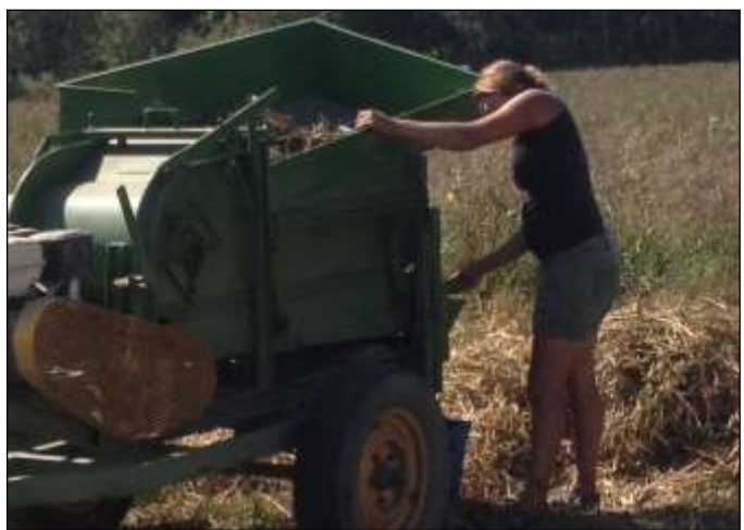
Figure 10. Portable bean thresher, Morningstar Meadows Farm, Glover, VT.
