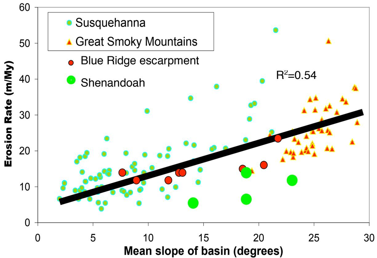
Figure 6: Plot of average basin slope vs.  $^{10}\text{Be}$  erosion rates for all available Appalachian data (Susquehanna from Reuter, 2005; Great Smoky Mountains from Matmon et al., 2003, Blue Ridge from my data; Shenandoah from Duxbury et al., 2006).
