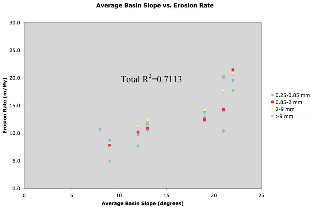
Figure 5: Plot of average basin slope vs. <sup>10</sup>Be erosion rates for all samples including grain size splits (size fractions designated  $\diamond=0.25-0.85$  mm,  $\square=0.85-2$  mm,  $\triangle=2-9$  mm,  $\times=>9$  mm).
