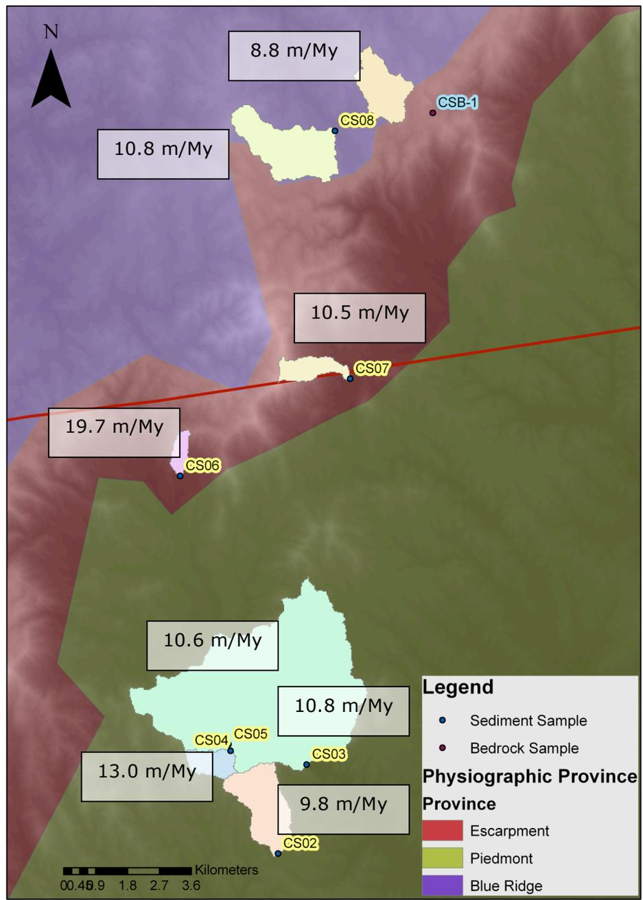
Figure 3: Transect C map of delineated basins and sample locations with modeled erosion rates (sand sized fraction only).
