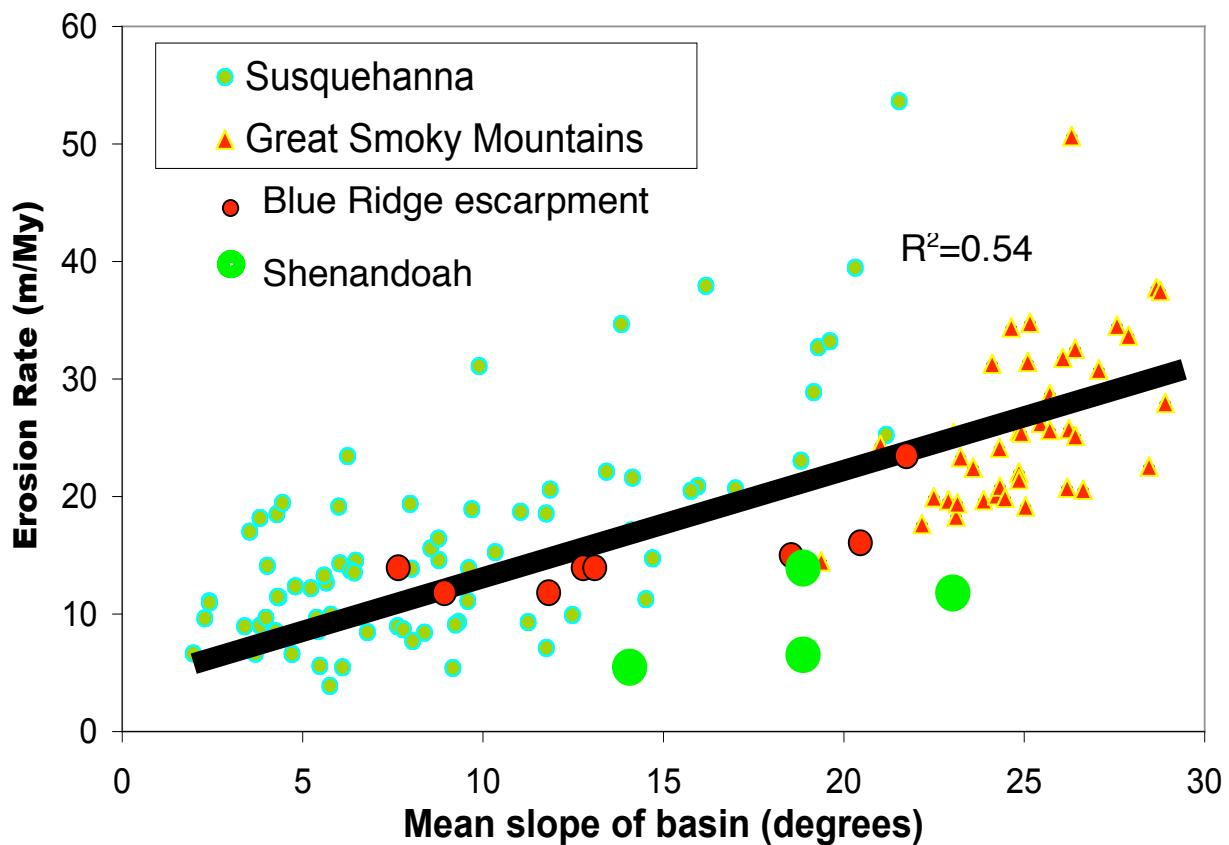
Figure 6: Plot of average basin slope vs.  $^{10}\text{Be}$  erosion rates for all available Appalachian data (Susquehanna from Reuter, 2005; Great Smoky Mountains from Matmon et al., 2003, Blue Ridge from my data; Shenandoah from Duxbury et al., 2006).
