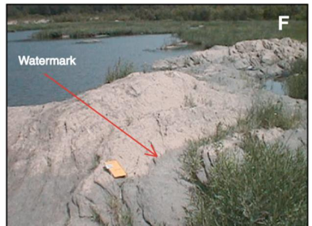
**F:** Picture shows the distinctive watermark used to determine the present river gradient in the upper gorge (mark could be correlated for approximately 2 km downstream). Field book for scale.
