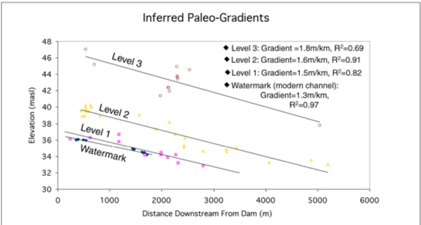
**Figure 6.** Inferred paleo-gradients for terraces levels 1, 2 & 3 derived from Trimble 4400 differential GPS data collected from all sample sites within the Holtwood Gorge field area in southeastern Pennsylvania. The Watermark trendline was constructed using GPS point of a distinctive watermark observed in the upper gorge (July, 2002). It is interpreted as being representative of the present river gradient.
