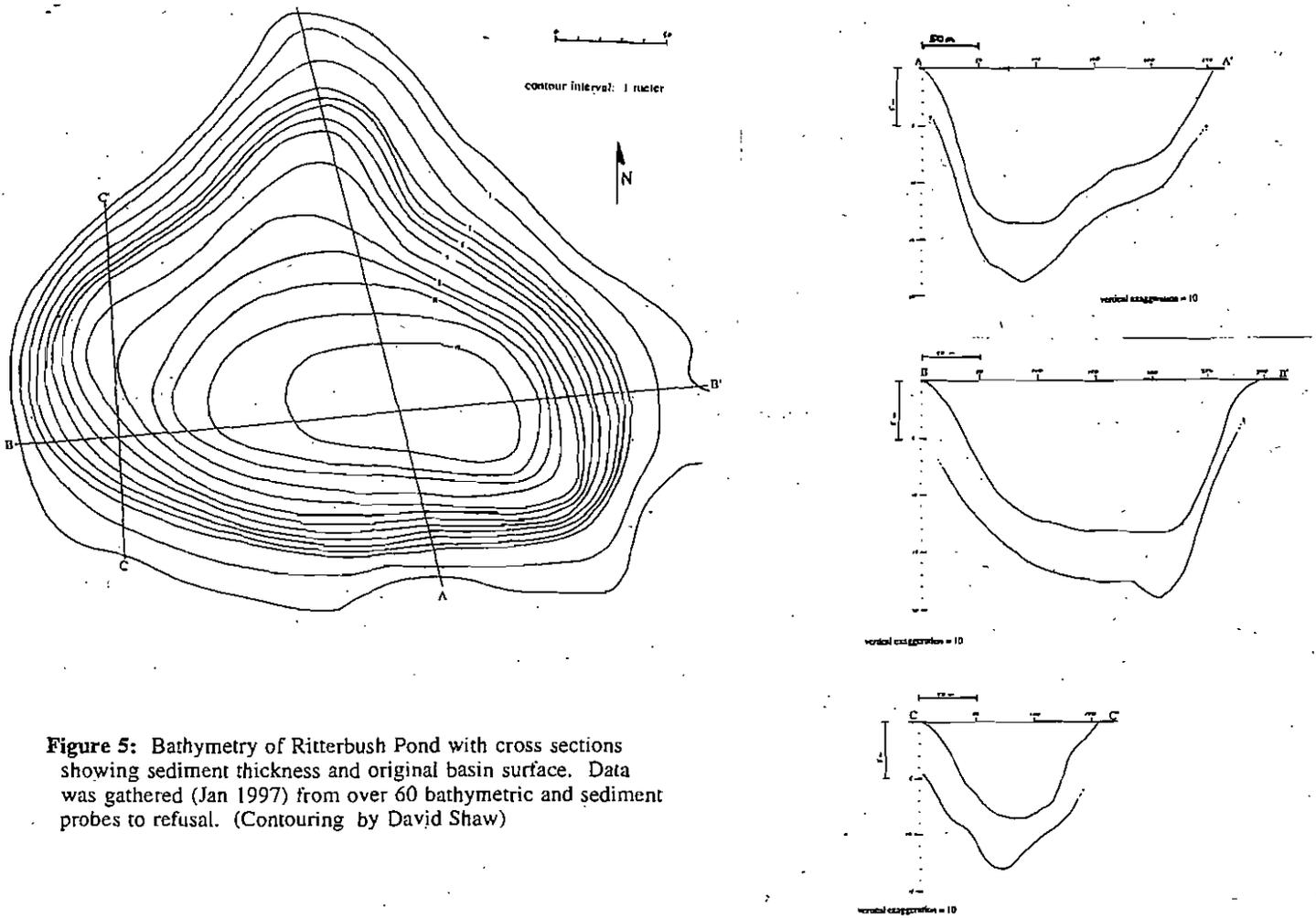
**Figure 5:** Bathymetry of Ritterbush Pond with cross sections showing sediment thickness and original basin surface. Data was gathered (Jan 1997) from over 60 bathymetric and sediment probes to refusal. (Contouring by David Shaw)
