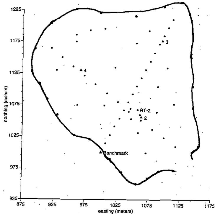
**Figure 6:** Data collected Jan - March 1997 at Ritterbush Pond. All points surveyed with electronic total station from the Benchmark on the lake perimeter. Bathymetric and sediment probe points are denoted by small dots. Core locations are marked by triangles. The approximate location of core RT-2 is also noted.
