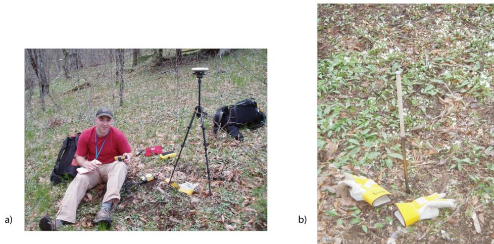
Figure 1. Field techniques from our recent round of fieldwork in the Great Smoky Mountains, TN. a) Trimble ProXH GPS unit setup for collecting 10-20 cm resolution GPS data for each soil pit on the Great Smoky Mountains hillslope. b) In addition to collecting GPS data, we drove a metal rod into the soil adjacent to each pit to determine the depth of the soil-bedrock contact.
