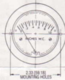
Dimensions, Series 2-5000 Minihelic II* Gage.
