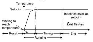
This is the same as mode 1 except that at the end of the timing period the controller will continue indefinitely in automatic control.
