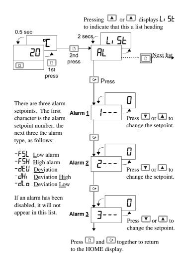
Note: The other parameters listed on pages 4 and 5 are accessed and adjusted in exactly the same way as this example.
