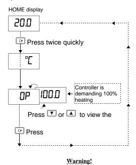
In manual standby mode (see 'To Use The Timer') the output power can be adjusted by the operator, causing heating or cooling to be permanently applied. To prevent this make the TP parameter read only (see 'To Hide, Reveal And Promote Parameters')
