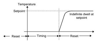
This mode applies a time delay before turning on the heating (or cooling). When the timer is started, the controller will always switch to standby mode and start counting down. When the timer has timed out, the controller will switch into automatic control, apply heating (or cooling) and control indefinitely at the setpoint.
