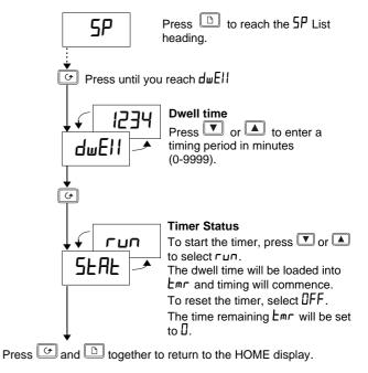
The 5EAE parameter can also be switched between DFF and run by configuring the logic I/O as a Off/run contact closure input.
