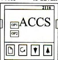
**Access List.** The Access list is used to enter the configuration mode as well as define mnemonic access levels. The Access list is password protected.
