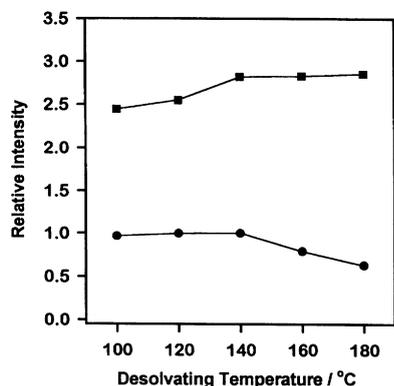
Fig. 2 Influence of mannitol on the emission signal of boron under different desolvating temperatures. Condensing temperature: 5 °C. &, Emission signal of 0.1 mg l<sup>-1</sup> B with 0.5% m/v mannitol; and \$, emission signal of 0.1 mg l<sup>-1</sup> B without mannitol.
