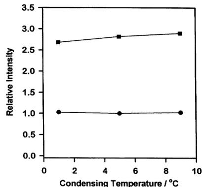
Fig. 3 Influence of mannitol on the emission signal of boron under different condensing temperatures. Desolvating temperature: 140 °C. &, Emission signal of 0.1 mg l<sup>-1</sup> B with 0.5% m/v mannitol; and \$, emission signal of 0.1 mg l<sup>-1</sup> B without mannitol.
