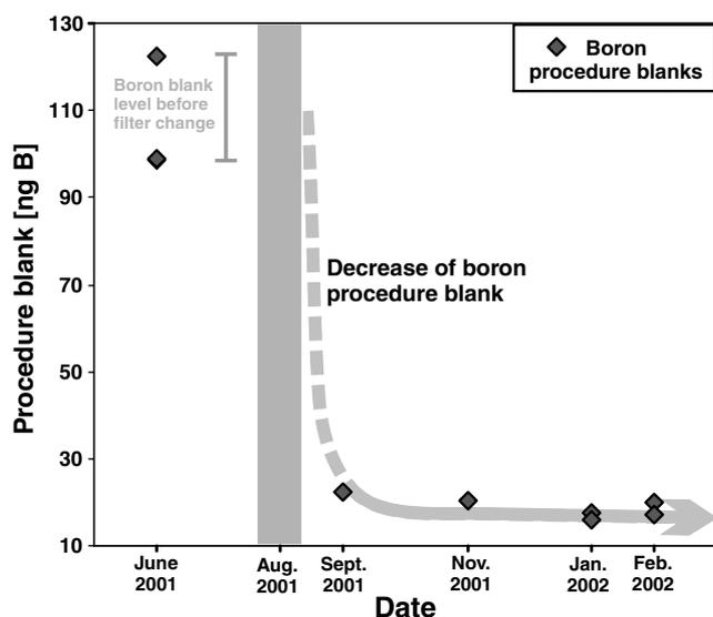
Fig. 3 Boron procedure-blank evolution before, to, and after the replacement of the boron-containing silicate glass pocket filters
