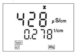
4 Set the cell constant to be used with  $\langle A \rangle \langle \nabla \rangle$ , e.g. 0.614 cm<sup>-1</sup>.
