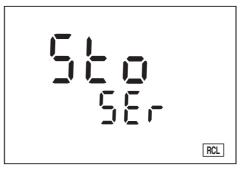
2 Press the **<RUN/ENTER>** key. The complete storage content is transmitted to the interface; during the data transmission the numbers of the currently transmitted storage locations run through. After the data transmission, the measuring instrument automatically switches to the measuring mode.
