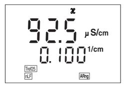
4 Set the cell constant to be used with  $\langle A \rangle \langle \nabla \rangle$ , e.g. 0.105 cm<sup>-1</sup>.
