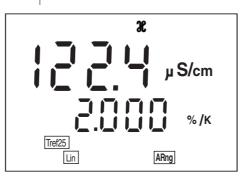
4 Set the temperature coefficient with  $< \blacktriangle > < \nabla >$ , e.g. 1.880 %/K.
