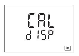
2 Press the **<RUN/ENTER>** key. The cell constant appears on the display, but the *CAL* display only appears when the displayed value was determined by calibrating the measuring cell.
