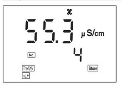
2 Confirm with **<RUN/ENTER>**. The display switches to entering the ID number.
