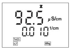
4 To return to the measuring mode: Press the  $\langle M \rangle$  key. From now on, the cell constant 0.010 cm<sup>-1</sup> will be used.
