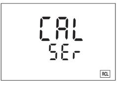
Press the **<RUN/ENTER>** key. The calibration protocol is transmitted to the interface. After the data transmission, the measuring instrument automatically switches to the measuring mode.
