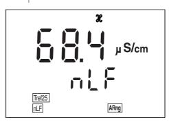
4 To return to the measuring mode: Press the **<M>** key. From now on, nLF will be used for the temperature compensation.
