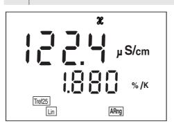
5 To return to the measuring mode: Press the **<M>** key. From now on, the adjusted linear temperature coefficient will be used for the temperature compensation.
