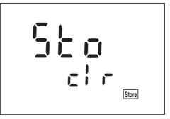
4 Confirm the clearing process with **<RUN/ENTER>**. Pressing any other key prevents the clearing, the data records will remain stored.
