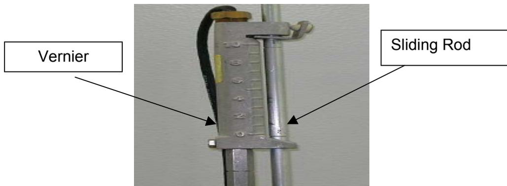
Figure 3. Top-Setting Wading Rod
