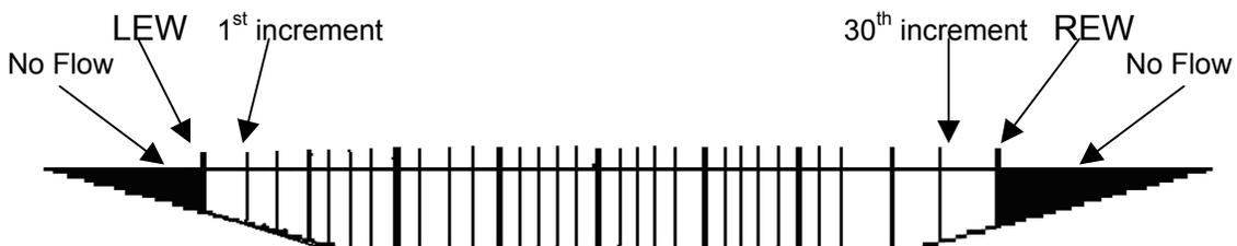
Figure 2. Stream divided into 30 increments
