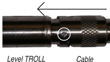
6. Grasp the knurled (textured) section of the cable connector in one hand and the Level TROLL body in the other. Push and twist firmly so that the pin on the body connector slides along the slot on the cable connector and locks securely into the other hole.
