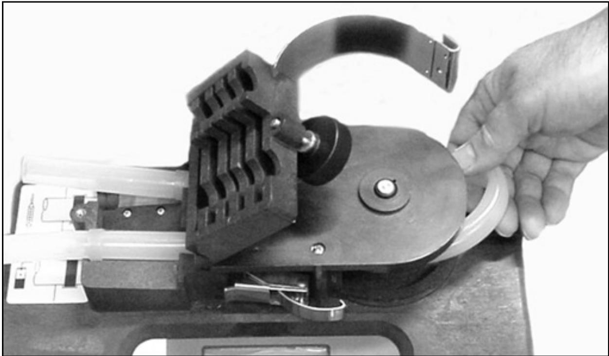
Figure 8-1 Removing and Replacing the Pump Tube
