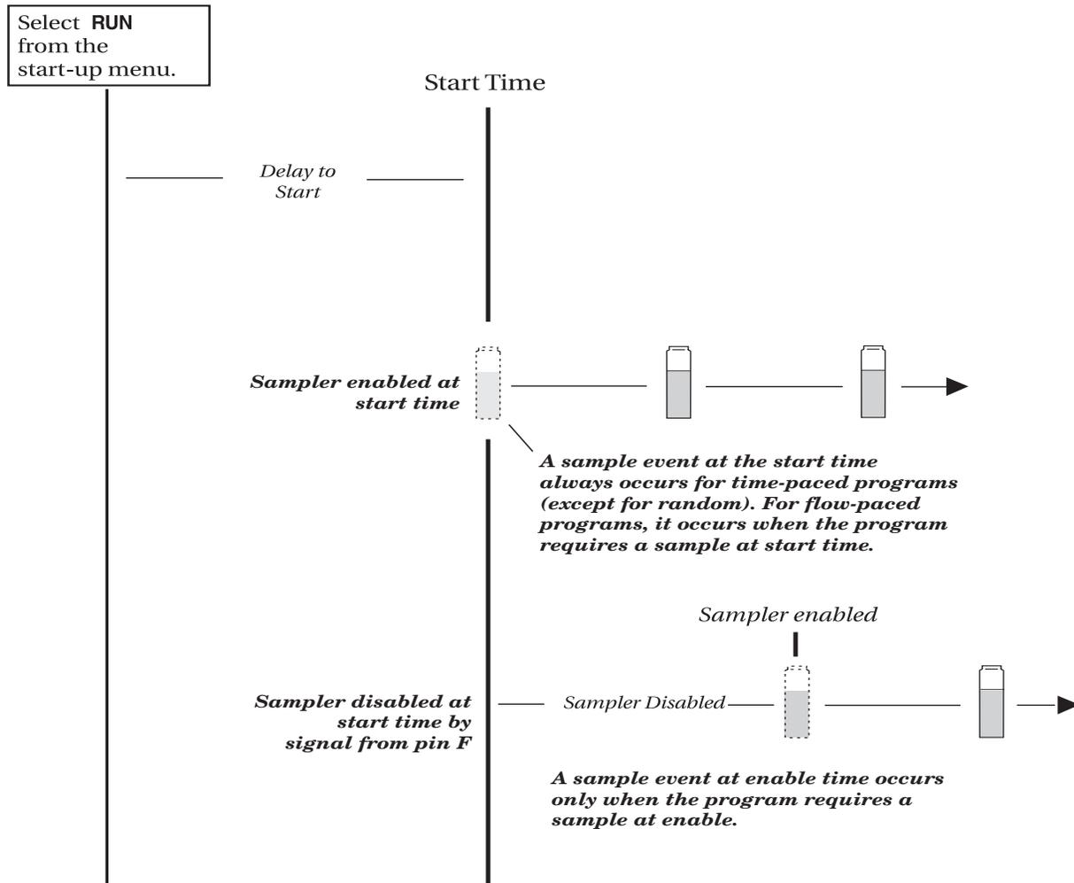
Figure 5-4 Start Time Diagram for Sampler Enable Settings
