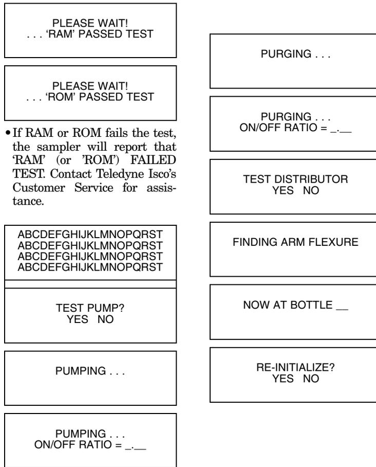
**Memory Test** – Screens 1 and 2 at left show you the diagnostic tests for the unit's memory. If either screen shows you a message saying that the memory failed the test, contact Teledyne Isco's Customer Service.
