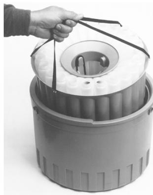
**Removing Bottles From the Compact Sampler**
