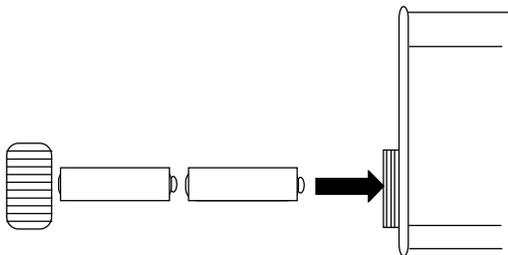
Twist the battery compartment cap clockwise, finger tight, to secure it.
