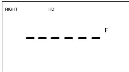
The indicator “RIGHT,” in the upper left quadrant of the screen, means you are using the right-hand button panel as your primary control panel.
