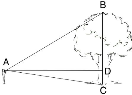
*Height measurement: The instrument first calculates AD, then measures angles CAD and DAB. It then calculates BD and DC. The height is the sum of BD and DC.*
