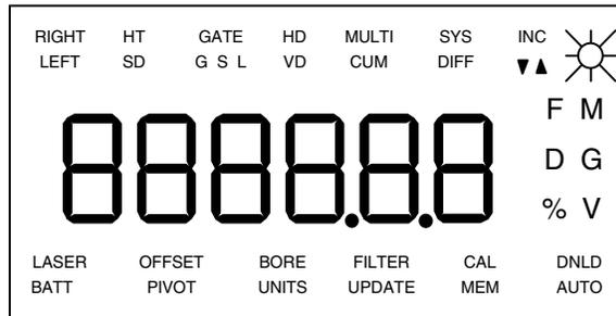
The display indicators are grouped by function, and fall into four categories: measurement modes, measurement modifiers, indicators/warnings, and settings/options. Note: Your instrument may not have all the features described.
