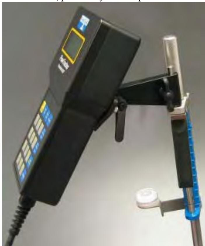
Figure 26 – Handheld Controller Mounting
