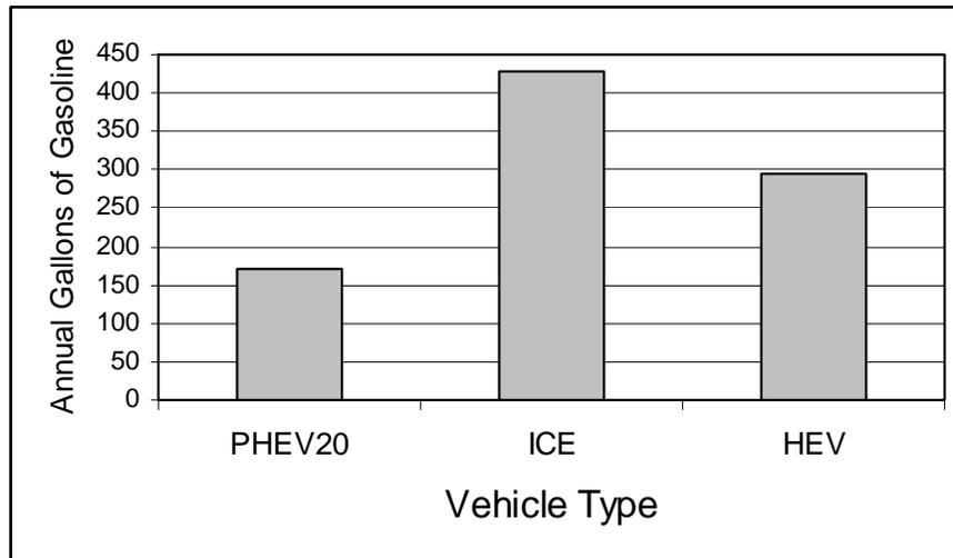
**Figure 14:** Annual Gasoline Consumption vs. Vehicle Type
