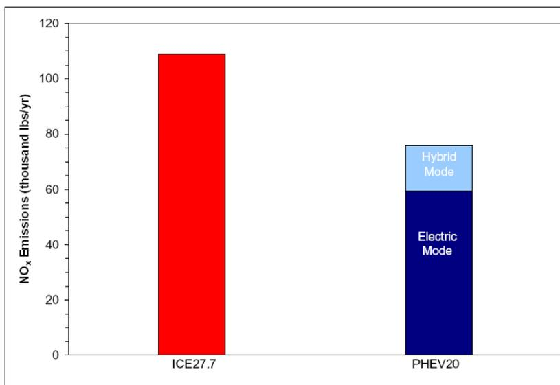
**Figure 13:** Annual NO<sub>x</sub> emissions from 50K ICE and 50K PHEV20 vehicles. It is assumed that each vehicle travels 12,379 mile annually.
