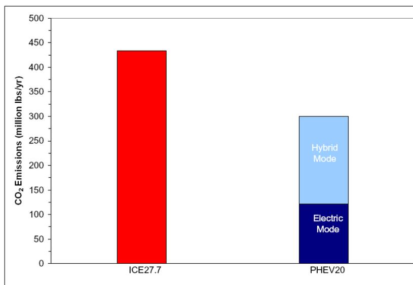
**Figure 12:** Annual CO<sub>2</sub> emissions from 50K ICE and 50K PHEV20 vehicles. It is assumed that each vehicle travels 12,379 mile annually.
