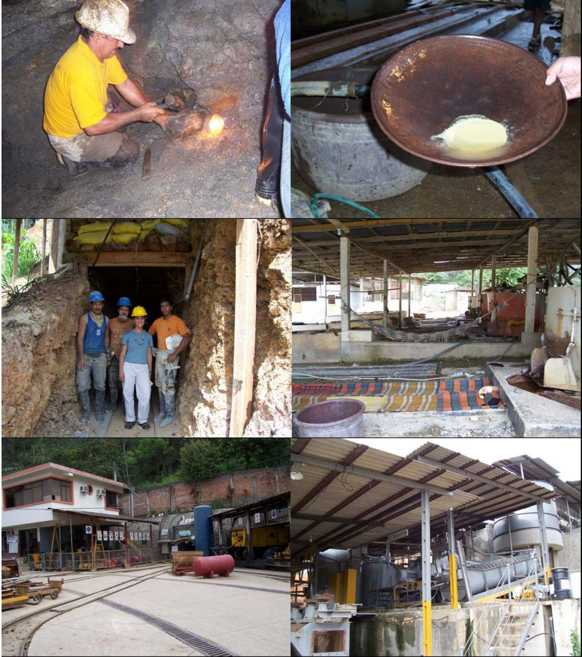
Figure 4. Scales of mining operations: top - artisanal, middle - small-scale semi-mechanized, bottom - small-scale industrialized
