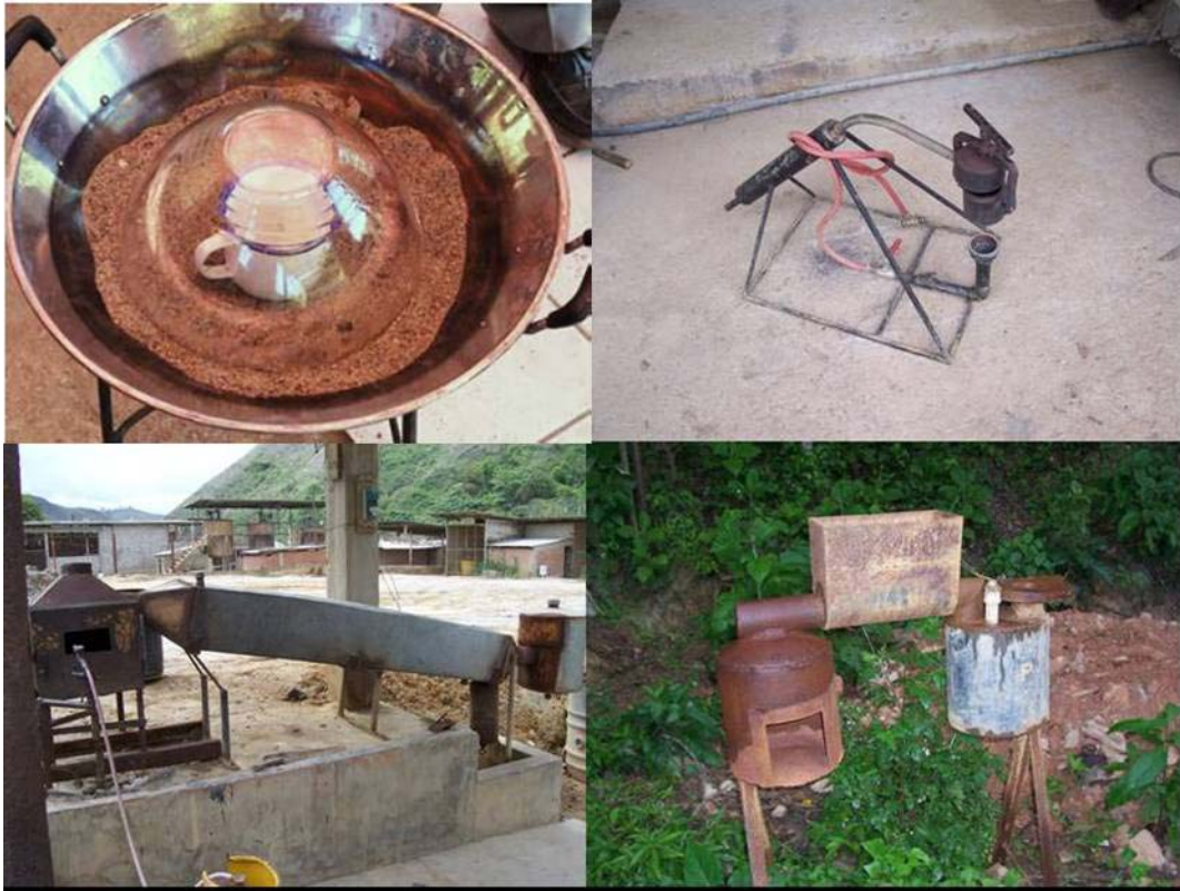
Figure 5: Examples of different retorts used in Southern Ecuador gold mining
