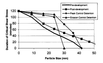
**Fig. 2.** Frequency and duration of critical shear-stress exceedence computed for four scenarios. Erosion control detention based on Meyer-Peter and Müller relationship using 8 mm gravel
