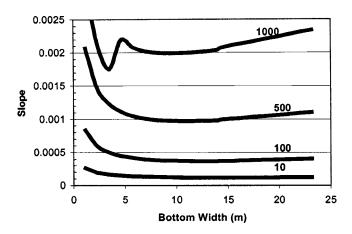
**Fig. 3.** Analytical stable channel solutions for sand-bed channels with different inflowing sediment concentrations. Solutions based on trapezoidal channel with 2:1 (*H*:*V*) bank angles, the Brownlie (1981) depth predictor and sediment-transport equations,  $Q = 10 \text{ m}^3/\text{s}$ , and  $d_s = 0.5 \text{ mm}$ . Note that upper curve depicts shift to upper regime bedforms at smaller widths occurring at that transport capacity
