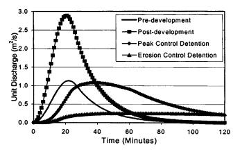
**Fig. 1.** Estimated Mail Creek unit discharge (2 year). Erosion control detention based on Meyer-Peter and Müller relationship using 8 mm gravel
